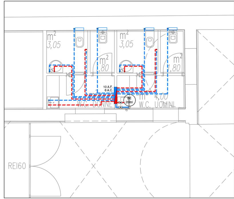
SCHEMA BOILER ELETTRICO E COLLETTORE SANITARIO
